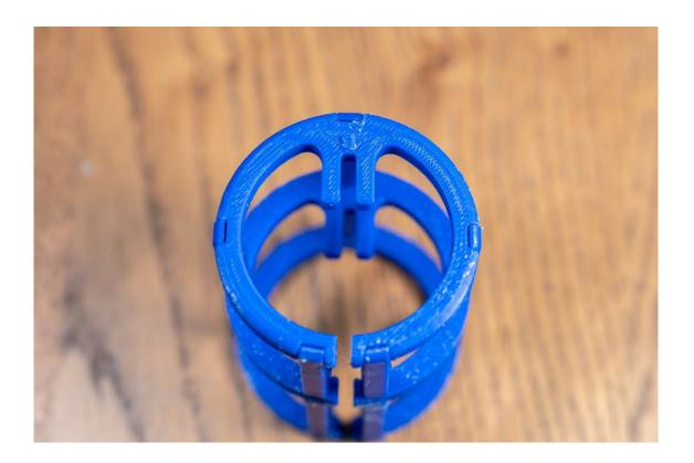
Once the eight frames are assembled, the snug onto the ORTF arms as shown below. Use some E6000 glue on the edge of the joint to lock it in place. Once all the glue is dry, you can slip on the actual furry wind screen.
